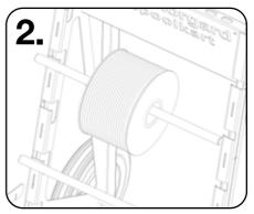
Slide the cable reels onto the loading bar and fit the loading bar back into place.
