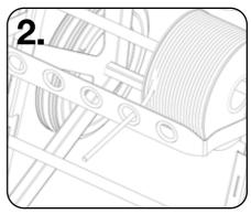
Pull cable through the feed bar in front of the reel. The feed bar helps prevent tangling, even when multiple cables are being used simultaneously.
