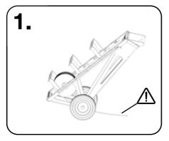
The loaded SpoolKart is easy to tilt and move to the desired location.
