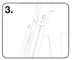
On the sides of the SpoolKart are measuring units to make it easy and simple to pull cable off in measured lengths.
