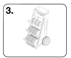
It's important that the load is spread evenly over the bars, with heavier reels on the lower bars. This will ensure the best stability of the SpoolKart.
