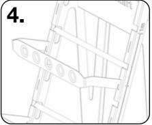
The feed bars work best when placed directly in front of the cable reels.
